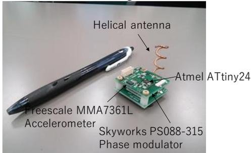
**Figure 11 MSMA sensor tag first prototype**
